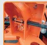
Leaf spring (for levelling the plough tilt)
