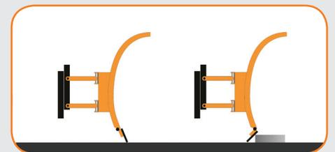
Protection with spring hatches allows the plough to clear obstacles of up to 100 mm.
